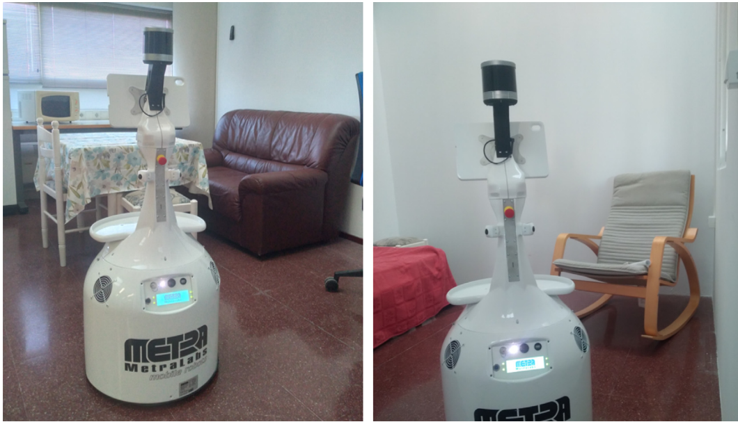
Fig. 13. The Morphia robot navigating in the small apartment.
